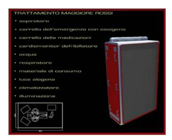
From this analysis of materials, it is evident that each unit requires "cases" of different dimensions, but, in order to define only one case to be used for all the functions, an ideal case size has been designed. The designed Case - inspired by the so-called flight-case used for the transport of fragile equipment and technologies - is made in extruded aluminium and includes anodised aluminium caps and details in ABS - Alkyl Benzene Sulfonate.
