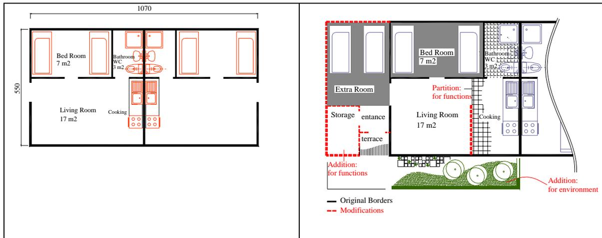
Figure 14 Initial design of temporary housing unit in Fevzi Çakmak Settlement adapted from Arslan (2004), drawn by author (2004) and Modified Units by residents: drawn by author
