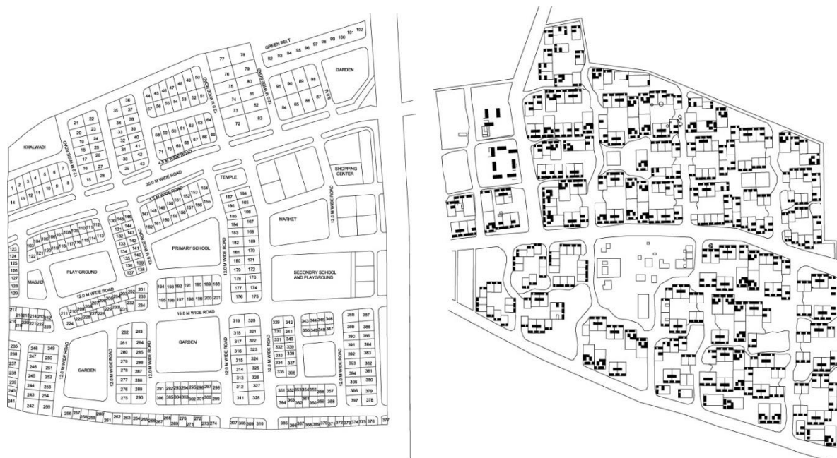
Figure 1: Left: relocated village of Sirsal's grid pattern layout; plan of 1996. Right: relocated village of Malkondji's cluster type layout; plan of 1996. Source: MEERP, 1996.
