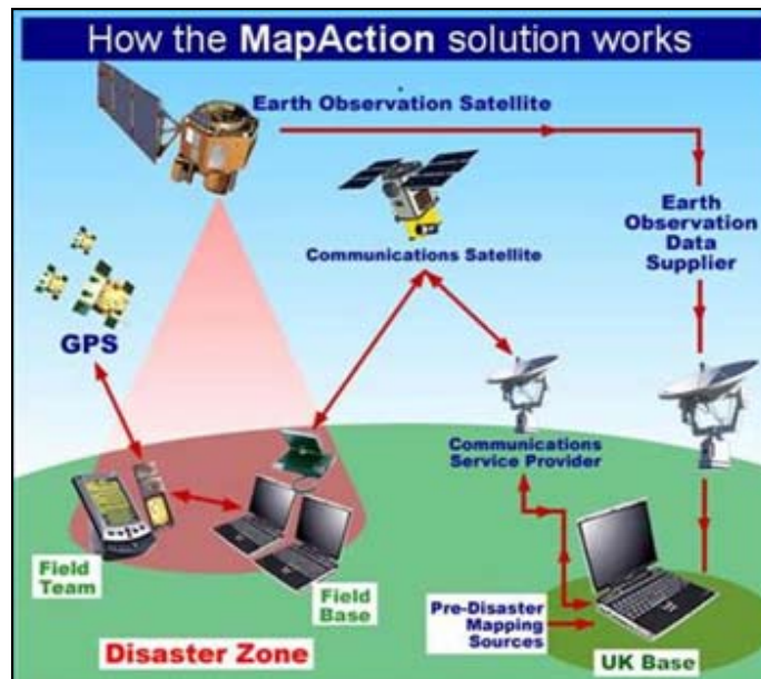
Fig. 2. Methodology Adopted by MapAction to Provide Real Time Mapping Capabilities Emergency Response Activities. (Technology Usage Diagram implemented by MapAction downloaded from www.mapaction.org )
